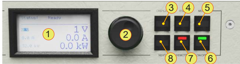
Fig. 91 Controls for the optional HMI (or the RCU).
