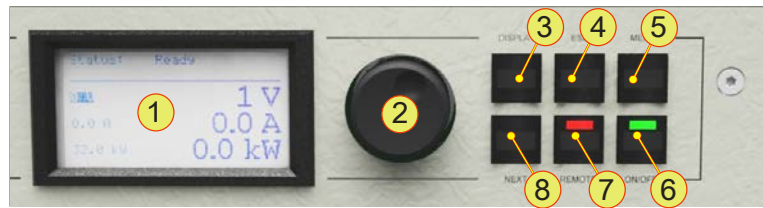
Fig. 10 Controls for the optional HMI (or the RCU).
