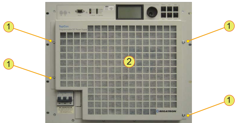
Fig. 115 The air filter mounting grille is fixed using 4 fastening screws.
