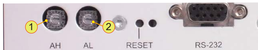
Fig. 82 Rotary switches AH -1- for the upper address range Rotary switch AL -2- for the lower address range
