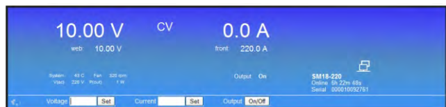
fig. 2 - 5, The front console of the web interface for setting of the input and monitoring various parameters.
