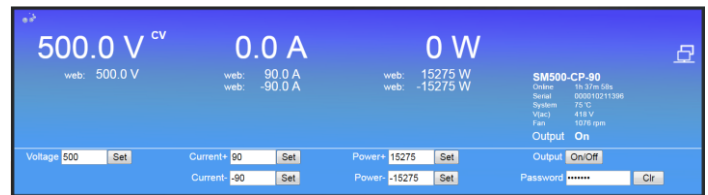
fig 4 - 4 - The front console of the web interface for setting of the output and monitoring various parameters.
