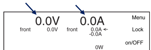
fig 6 - 15 The first line in the display shows the actual output value for voltage and current.
