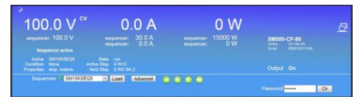
fig 8 - 2 Sequencer console for selecting and controlling sequences.
