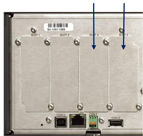
fig 4 - 1 Slot 3 and 4 are valid for INT MOD M/S-2.
