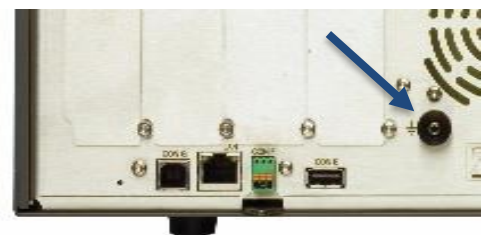
fig 4 - 4 Use this M4-size bold for connecting al CBL2603.
