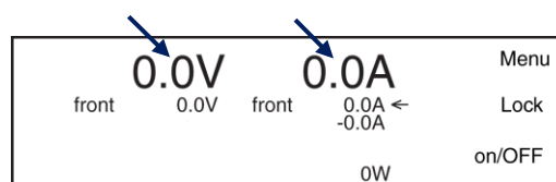
fig 6 - 16 The first line in the display shows the actual output value for voltage and current.
