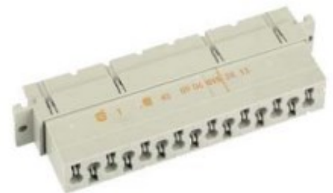
Figure 8. H15 Cage Clamp type female - H15-CC The cable rating is AWG16 or <1.5 \text{ mm}^2 . That makes it not usable for 24T-input and 5 V outputs.
