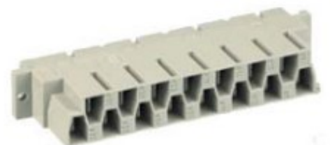
Figure 9. H15 FastOn 6.3 mm female - H15-T The TABS are rated 12 A 70°C or 15 A 55°C thus 2.5 \text{ mm}^2 or AWG13
