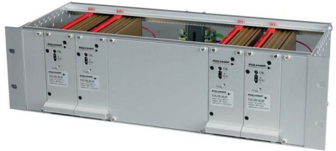
At high DC input or output voltages e.g. 110 Vd.c. "Hot plug-in" is not recommended, due to arcing on the connectors. The photo and figure 3 above is an example of Safety Critical power supply system where 2 different input batteries are used (A and B) with 2 or 3 redundant units per group. All outputs are parallel connected with alarm signalization. One side can also be supplied by AC.
