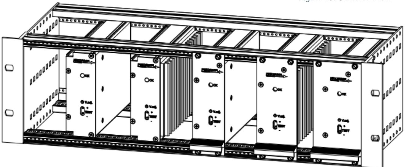
Figure 11. PSC mounted in Euro format 19"-subrack without TE panel. The type code do not include the letter L (L-panel)
