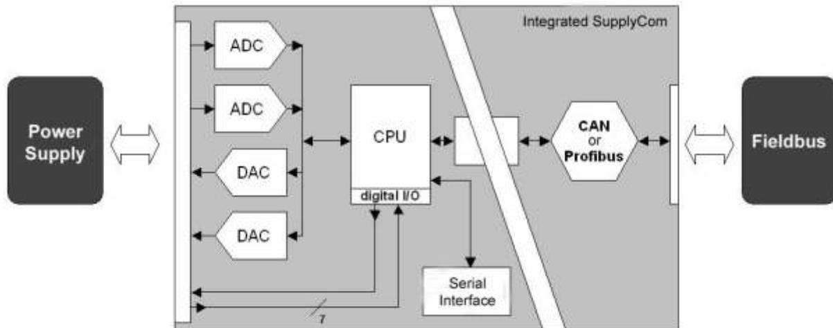
fig. 1 - Function diagram of the Integrated SupplyCom
