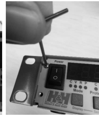
Figure 7.7: Assembling the left brackets
