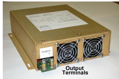
Figure 5 LDY Output Connections
