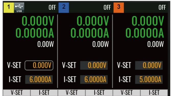
Triple-Channel Meter Interface and Quick Setup Interface
