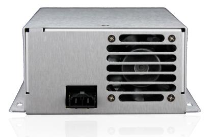
The HPP-750 laser diode pulser is a new concept in pulsed diode driver development. Designed to be used with the LDD series drivers as the power source, the HPP-750 pulser can deliver up to 350 amps of output current with full protection of the laser diode. Pulse widths of  $\geq$ 50µs to CW can be acheived with rise/fall times of <10µs. and repetition rates to 5kHz.
