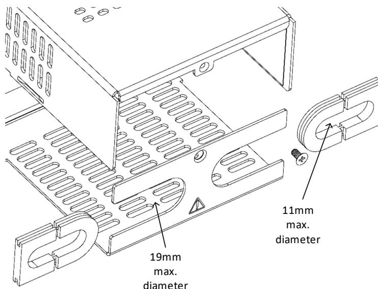
**Figure 4-36: Bus bar Cover Wire Diameter Limitation**
