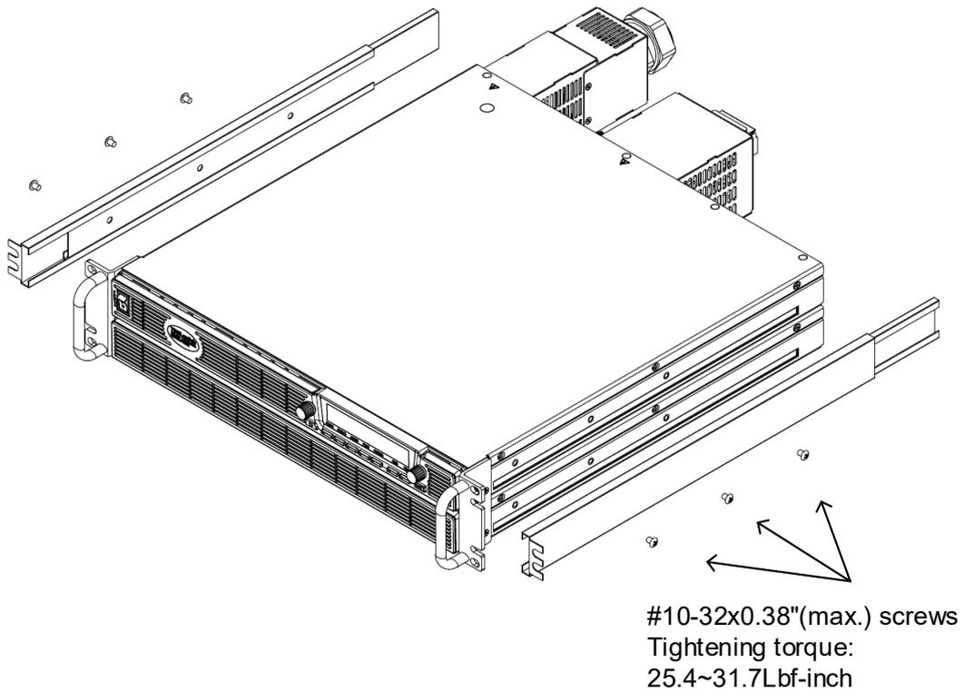
**Figure 4-13: 10kW Rack – Mount Slides Assembly**
