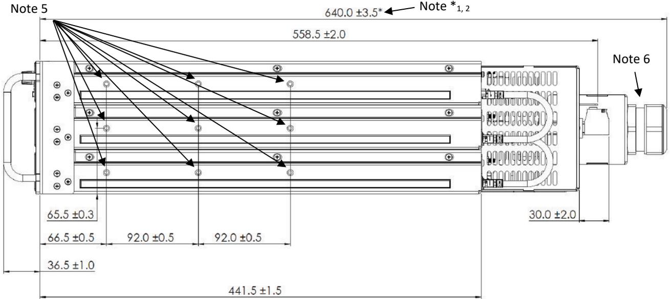
**Standard & Blank Panel Units Side View (10V ~ 100V):**
