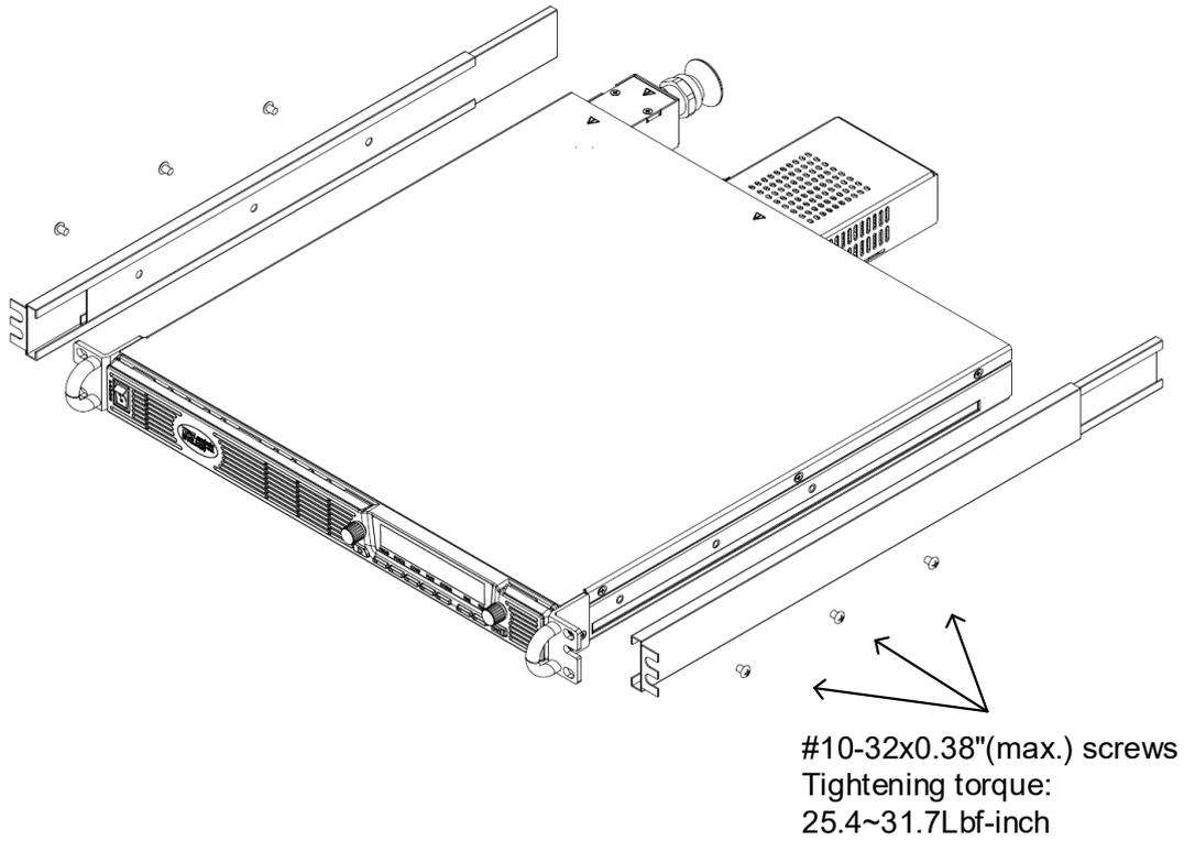
**Figure 4-12: 1 - 5kW Rack – Mount Slides Assembly**
