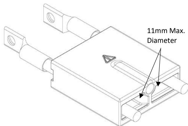
**Figure 4-35: Bus Bar Cover Wire Diameter Limitation (Half Width Models)**
