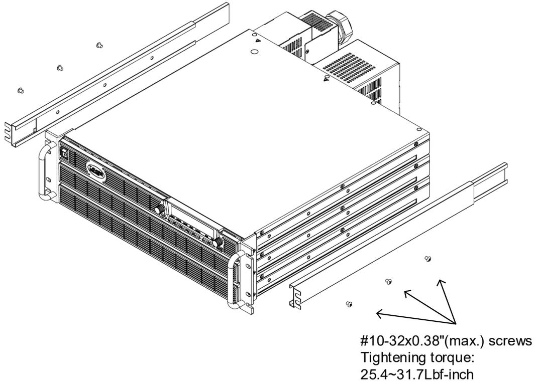
**Figure 4-14: 15kW Rack – Mount Slides Assembly**
