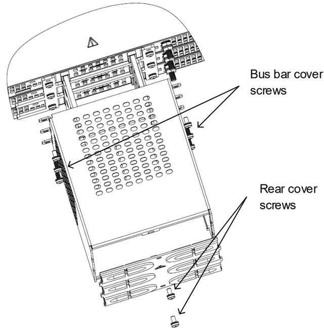
**Figure 4-54: Disassembly of Output Protection**
