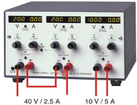
fig. 3 - 3 Series Tracking Mode
