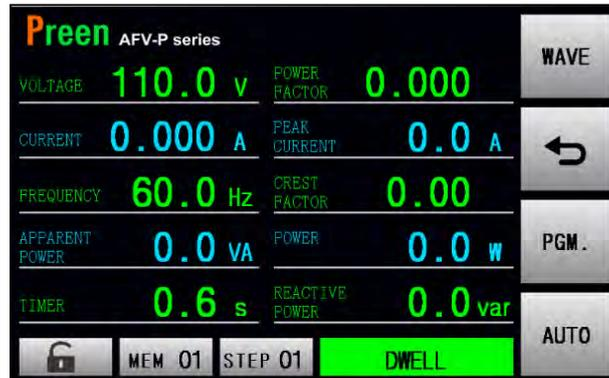
Figure 3.53 METER page when the PROGRAMMABLE feature is performed
