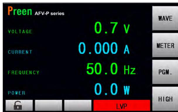
Figure 3.20 The MAIN page when LVP is triggered
