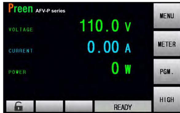
Figure 3.12 MAIN page when the output mode is DC
