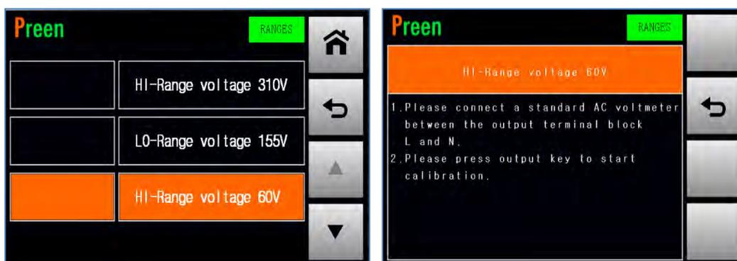
Figure 6.9 Enter into the page which calibrates the HI-Range voltage 60V
