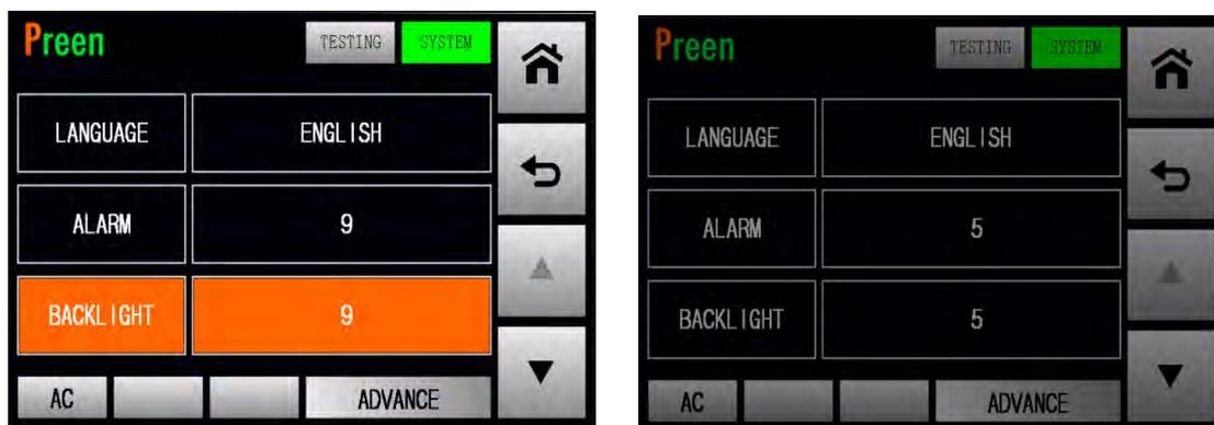
Figure 3.38 Set the backlight level from 9 to 5
