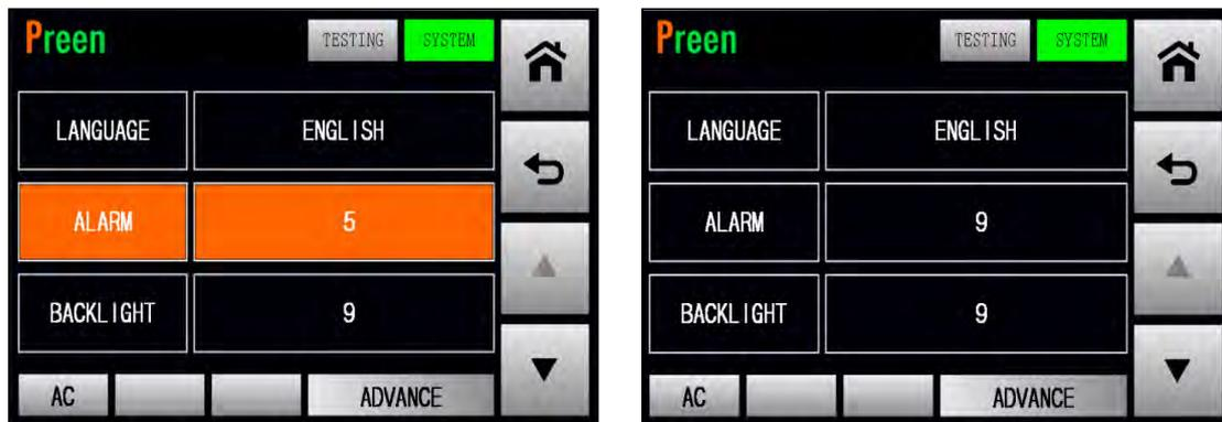
Figure 3.37 Set the alarm volume from 5 to 9
