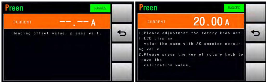
Figure 6.21 Enable the calibration of the output socket current
