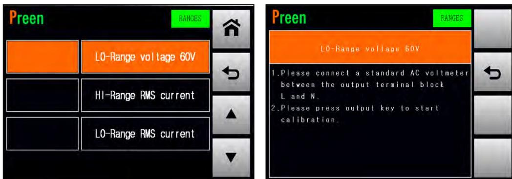
Figure 6.11 Enter into the page which calibrates the LO-Range voltage 60V
