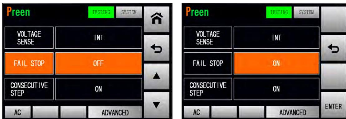
Figure 3.21 Enable the fail stop feature (ADVANCED mode)
