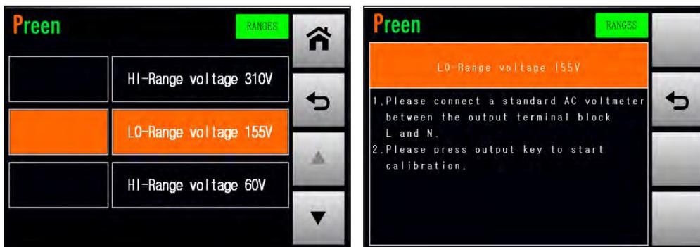
Figure 6.7 Enter into the page which calibrates the LO-Range voltage 155V
