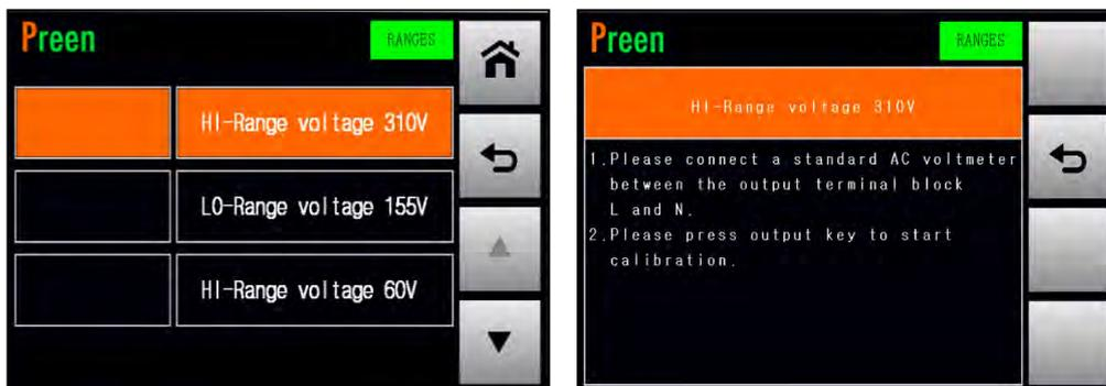
Figure 6.5 Enter into the page which calibrates the HI-Range voltage 310V
