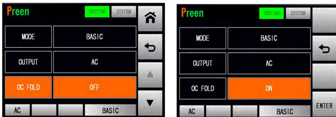
Figure 3.28 Enable the OC-FOLD mode (BASIC mode)
