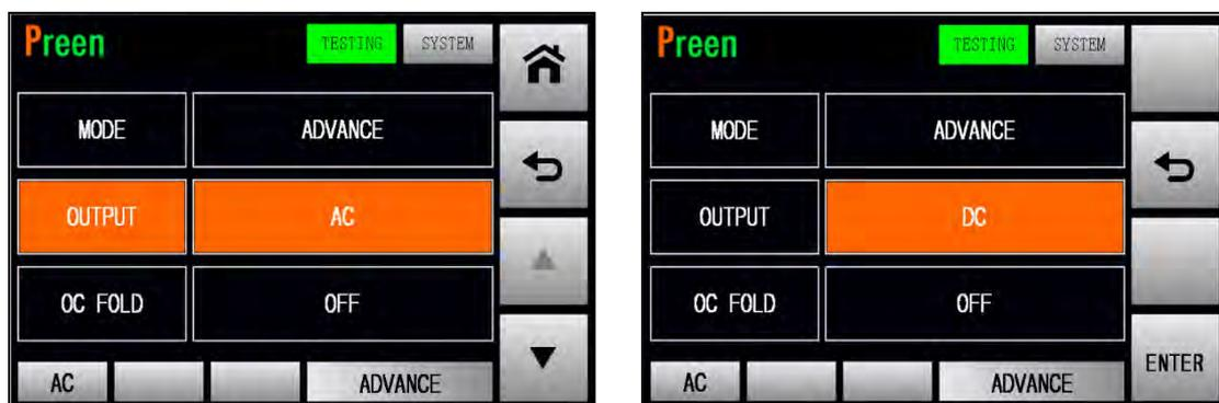
Figure 3.13 Set the output mode from AC to DC (ADVANCED mode)
