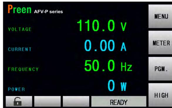
Figure 3.11 MAIN page when the output mode is AC
